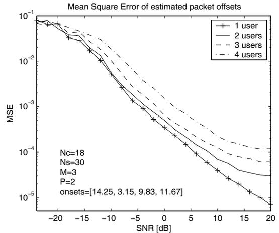
Figure 4: Mean square error of the correctly estimated packet offset delays.
