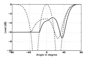
Figure 1: Beampattern of g(t) (solid line) and impulse g(t) (dashed line) arriving at 90° on array  $1_2$  with 2 elements at distance and of narrowband signal with wavelength (dash-dotted)
