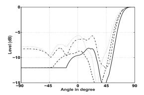
Figure 7: Beampattern of g(t) (solid line) and impulse g(t) (dashed line) arriving at  $90^{\circ}$  on array  $1_4$  with 4 elements at distance and of g(t) (dash-dotted line) and impulse g(t) (dotted line) on array 1 with different prefilters
