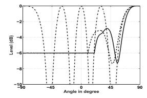
Figure 2: Beampattern of g(t) (solid line) and impulse g(t) (dashed line) arriving at 90° on array  $2_2$  with 2 elements at distance 2 and of narrowband signal with wavelength (dash-dotted)
