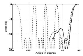
Figure 4: Beampattern of g(t) (solid line) and impulse g(t) (dashed line) arriving at 90° on array 24 with 4 elements at distance 2 and of narrowband signal with wavelength (dash-dotted)
