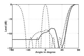
Figure 3: Beampattern of g(t) (solid line) and impulse g(t) (dashed line) arriving at 90° on array  $1_4$  with 4 elements at distance and of narrowband signal with wavelength (dash-dotted)
