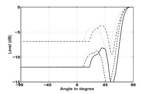
Figure 6: Beampattern of g(t) (solid line) and impulse g(t) (dashed line) arriving at  $90^{\circ}$  on array  $2_4$  with 4 elements at distance and of g(t) (dash-dotted line) and impulse g(t) (dotted line) on array 1 with Hamming shading
