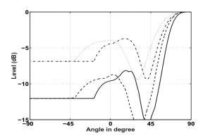
Figure 5: Beampattern of g(t) (solid line) and impulse g(t) (dashed line) arriving at 90° on array 14 with 4 elements at distance and of g(t) (dash-dotted line) and impulse g(t) (dotted line) on array 1 with Hamming shading
