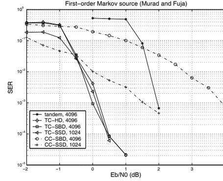
Figure 4: Comparison, after three iterations, of symbol error rates for the first-order 3-symbol Markov source with VLC encoding and with  $32 \times 32$  and  $64 \times 64$  block interleavers.
