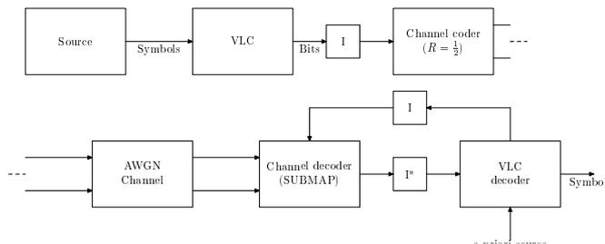
Figure 2: Iterative decoding scheme between source and channel for the JSCD of VLC.
