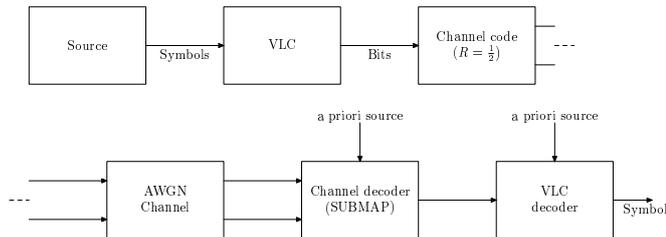
Figure 1: Source-controlled turbo decoding of VLC using *a priori* source information.
