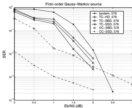
Figure 5: Comparison, after three iterations, of symbol error rates for the Gauss-Markov source with a 16-level quantizer, VLC encoding and a  $24 \times 24$  block interleaver.
