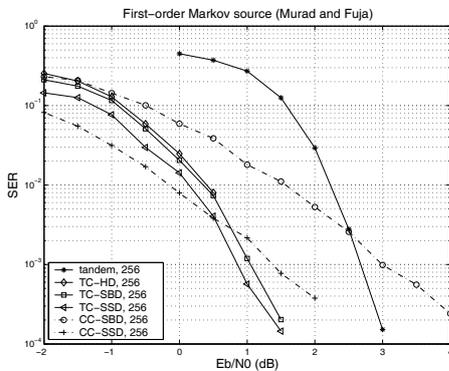
Figure 3: Comparison, after three iterations, of symbol error rates for the first-order 3-symbol Markov source with VLC encoding and a  $16 \times 16$  block interleaver.
