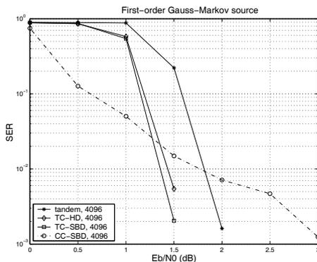
Figure 6: Comparison, after three iterations, of symbol error rates for the Gauss-Markov source with a 16-level quantizer, VLC encoding and a  $64 \times 64$  block interleaver.
