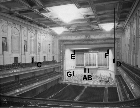
Figure 1: An example of how microphones may be arranged in a recording venue for a multichannel recording.
