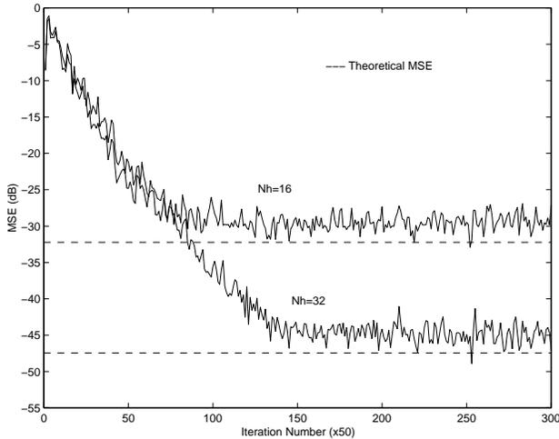
**Fig. 3.** MSE evolution of the overdetermined subband structure of Fig. 1 with colored input.
