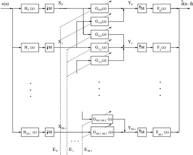
**Fig. 1.** Overdetermined adaptive subband structure with critical sampling [3].
