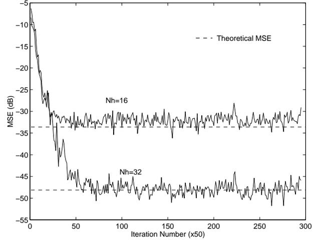
**Fig. 4.** MSE evolution of the non-overdetermined subband structure of Fig. 2 with colored input.
