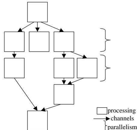
Figure 2: Example of structure proposed by DK1 tool. Some parallel functions can be achieved; the second line indicates a parallelism between 3 functions (DK1 tool manages all synchronisations). Data is transferred by means of channels
