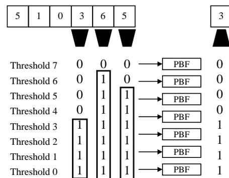
Figure 5: Example of stack filter. The 3bits input sample is threshold in 8 levels ( $=2^3$ ). Then, a series of PBFs computes the min value for each level. The result is a stack of '1' and '0' representing the output sample.
