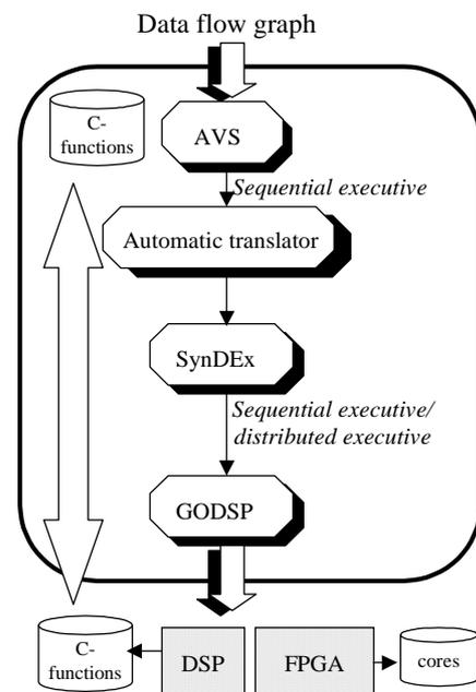
Figure 1: Rapid prototyping process for implementation of image processing applications.
