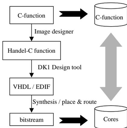
Figure 4: Process of core generation with DK1 tool.
