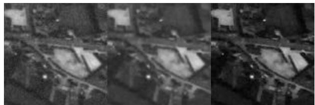
Figure 2 : (a) Band 3: degradation model 4,  $\sigma_{noise}=8$ , (b) After filtering (additive,  $\sigma_{noise}=10,64.$ ), (c) After restoration.
