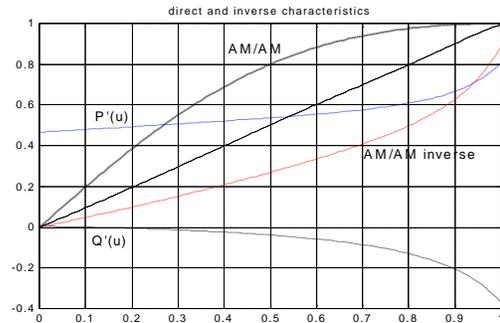
Figure 6: Direct (theoretical) and estimated inverse non-linear characteristics.  $P'(u)$  and  $Q'(u)$  curves (eq. ) and linearization.
