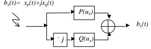
Figure 1: Quadrature nonlinear model of HPA.
