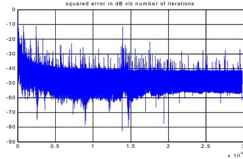
Figure 5: Evolution of the LMS squared error in dB.
