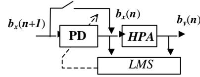
Figure 4: Block diagram of the adaptive pre-distortion.
