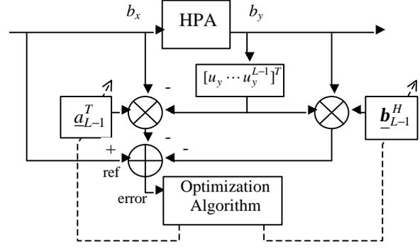
Figure 3: Block diagram of the system identification problem for the HPA's base-band model.
