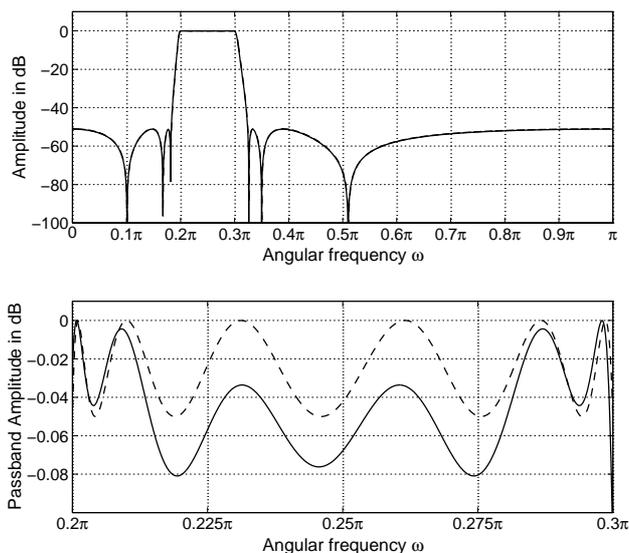
Fig. 3. Amplitude responses for the infinite-precision BPF filter with stricter criteria (dashed line) and for the filter with forty-eight nonzero bits (solid line).
