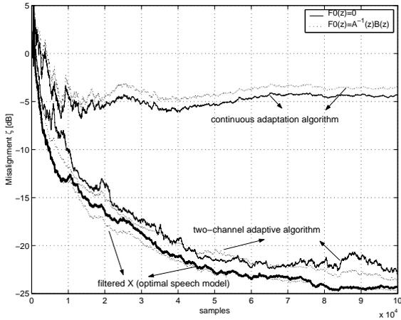
Figure 4: Frequency domain misalignment  $\zeta(F, \hat{F})$  of the feedback path estimate  $-A^{-1}(z)B(z)$  for  $d = 11$ .
