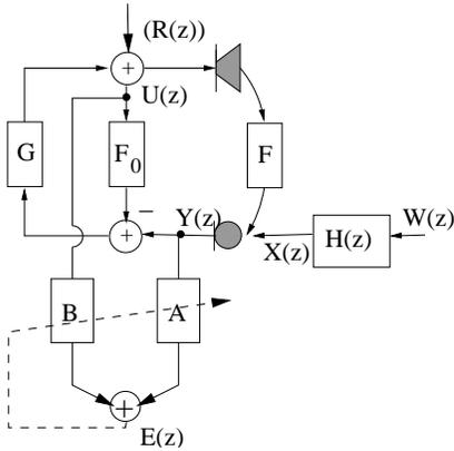
Figure 3: Two-channel identification scheme.
