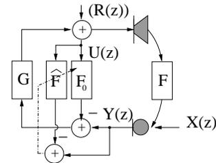
Figure 1: Concept of a (biased) adaptive feedback canceller.
