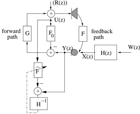
Figure 2: Filtered-X algorithm.
