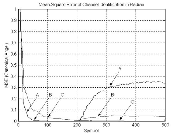
Fig. 1. MSE of Channel Identification in impulse noise
