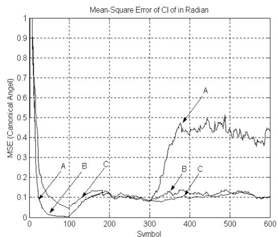
Fig. 3. MSE of Channel Identification in slow time-varying channel
