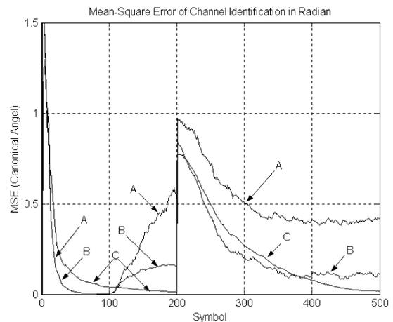
Fig. 2. MSE of Channel Identification in sudden change channel
