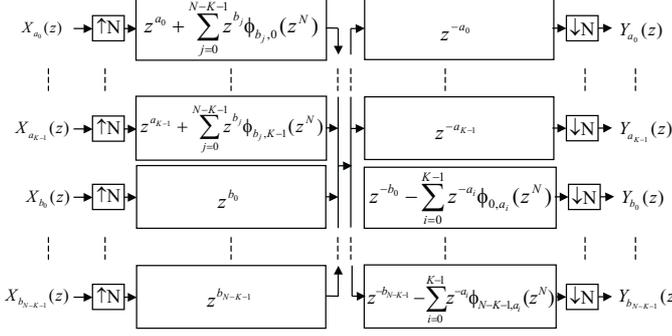
Figure 3: Extended  $N$  channel perfect reconstruction transmultiplexor.
