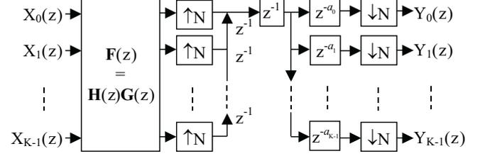
Figure 6: Polyphase representation of the transmultiplexor core of the proposed system.
