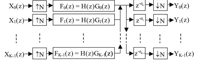
Figure 5: Transmultiplexor core of the proposed system.
