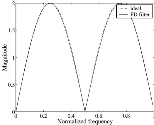
Fig. 4. The frequency response of the comb stage with the ideal delay, and non-integer delay filter.
