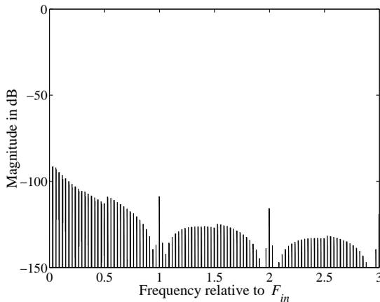
Fig. 5. Aliasing bands of the overall structure.
