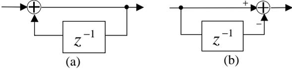
Fig. 1.(a) Integrator filter. (b) Comb filter.
