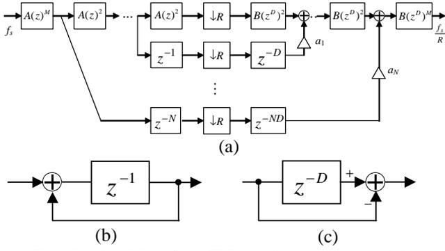
Fig. 3. (a) Modified CIC with non-integer delay. (b) Integrator filter with transfer function  $A(z)$ . (c) Comb filter with transfer function  $B(z)$ .
