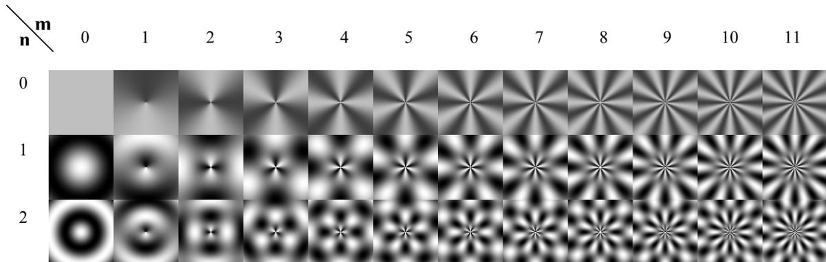
Figure 1. Real parts of ART basis functions (N=3, M=12).
