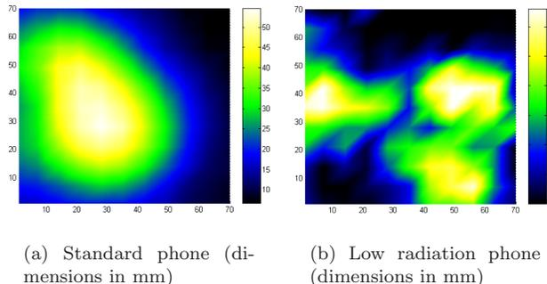
Fig. 3: Total E-Field in a plane in the head-phantom, at 1800 MHz.
