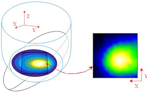
Fig. 4: Representation of the ellipsoidal model of the electric field, inside the phantom, with the data acquisition plane. The real cut shown at the right is issued from a real measurement.
