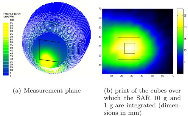
Fig. 2: Total E-Field in the head-phantom, at 1800 MHz.
