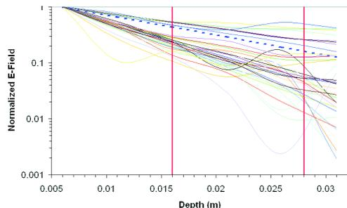
Fig. 1: Depth decrease of the maximum normalized E-Field, for 40 phones at 1800 MHz. The dotted line represents the decay of the theoretical plane wave in the same propagation medium. Vertical lines represent the limits in depth of the 1 g (left) and 10 g (right) averaging volume.
