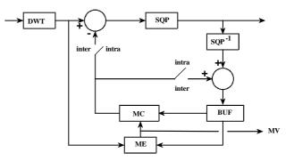
Figure 1. Wavelet based video encoder without inverse discrete wavelet transform.
