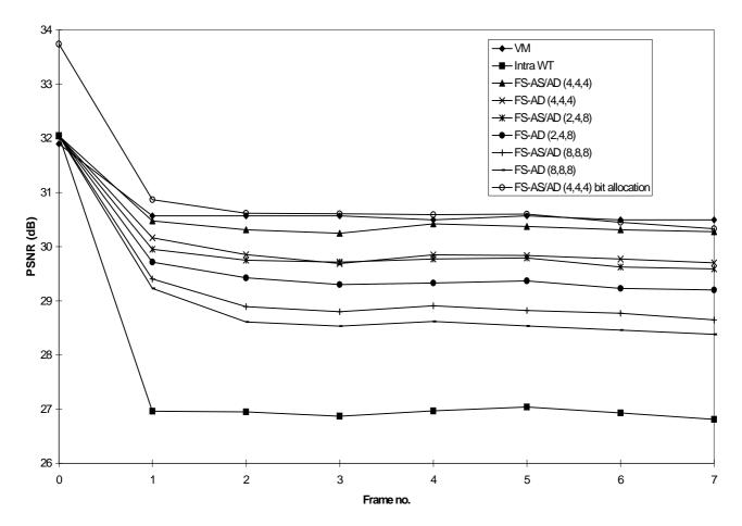
Figure 4. Coding results of the wavelet video encoder, using FS-AS/AD or FS-AD, and the MPEG-4 Verification Model (VM) for the "Mobile & Calendar" sequence. Intra wavelet coding of all frames is also indicated.
