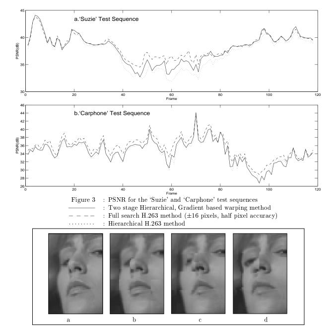
Figure 4: Reconstructed Frame 50 (a) Original (b) Full search H.263 (c) Hierarchical H.263 (d) Two-stage scheme
