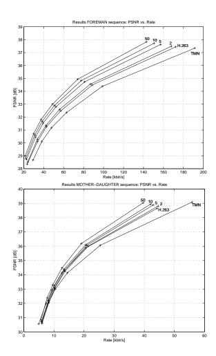
Figure 2: PSNR vs. overall bit-rate for the sequences *Foreman* (top) and *Mother-Daughter* (bottom). The quantization parameter is varied over the values 7, 10, 3, 16, 22, and 31.
