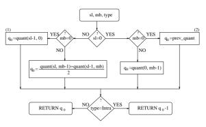
Figure 3: Algorithm scheme for the calculation of the quantization factor  $q_0$ .
