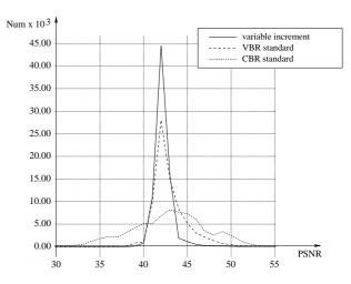
Figure 7: PSNR histogram of the coded macroblocks with 42 dB target.
