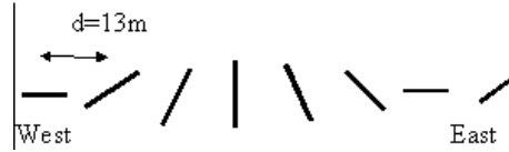
Figure 1: Linear heterogeneous array of equi-spaced antennas
