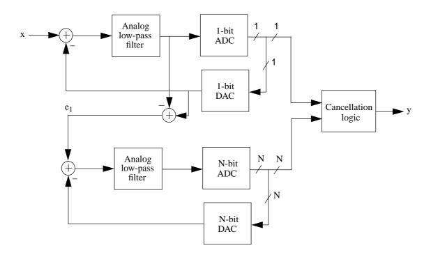
Figure 5. A cascaded  $\Delta\Sigma$  modulator
