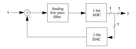
Figure 4. An analog noise shaping loop
