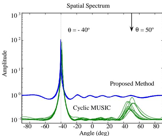
Figure 2 The spatial spectra of the DOA estimation of the AM signal by using the cyclic MUSIC and the proposed method with  $\alpha = 0.4$ .
