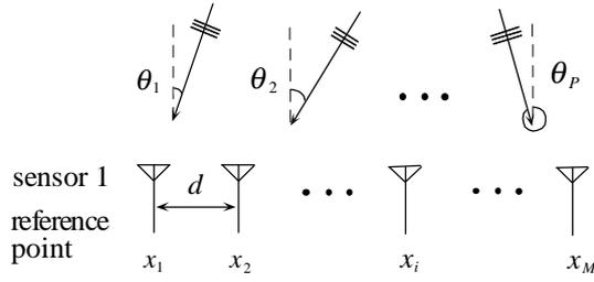
Fig. 1 The structure of a uniform linear array.
