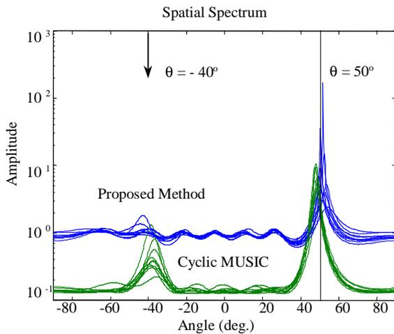
Figure 1 The spatial spectra of the DOA estimation of the BPSK signal by using the cyclic MUSIC and the proposed method with  $\alpha = 0.25$ .
