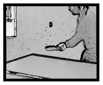
Figure 4: Vectors discarded during the robust regression phase (marked in black and overimposed to original frame).
