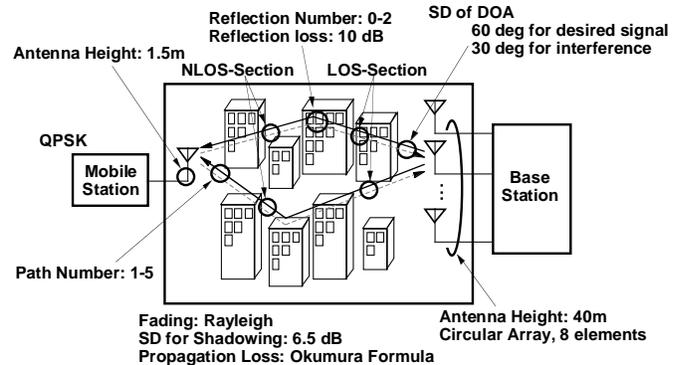
Fig. 2 Propagation Conditions
