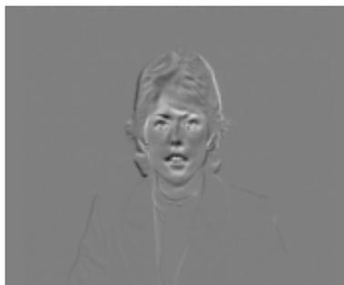
Figure 7: Frame difference between original frames 0 and 2 for "Claire".
