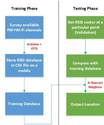
Fig. 1: Flow diagram of the proposed system
