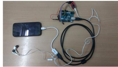
Fig. 2: Experimental Setup: Si-4703 FM Radio Receiver connected to a Moto G smartphone using an Arduino Uno and an OTG cable.
