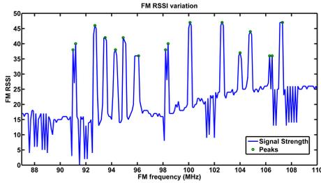
Fig. 3: Typical plot of FM RSSI measurement: Peaks identified before processing are shown with circles. Peaks very close to each other correspond to the same FM station.
