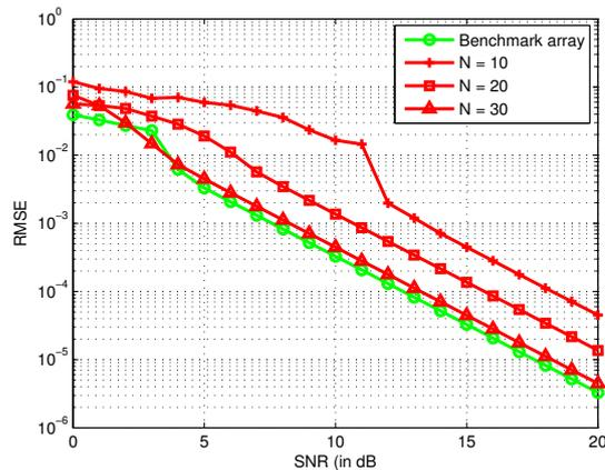
Fig. 4. Comparison of RMSE vs SNR for the reconstructed spectrum for different delay channels and the benchmark array.
