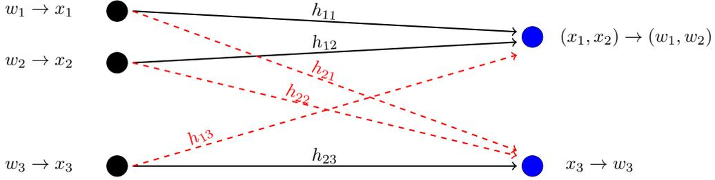
Fig. 2: A Partial Interference Multiple Access Channel (PIMAC). The transmit signals  $x_j$  are a function of the messages  $w_j$  which are the realizations from the Gaussian codebook.
