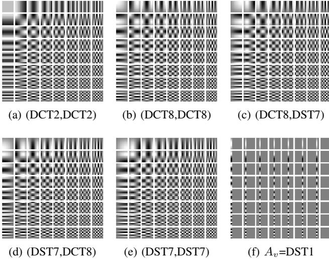
Fig. 1: 8x8 Transform basis of 2D-transforms used in the proposed systems. The five first transforms are used in the transform set containing 5 transforms. (f) represents the 2D-transforms (T7) when only the DST1 acts in the vertical direction.
