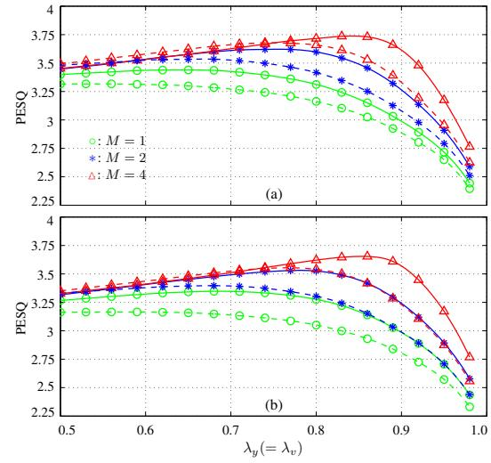
Fig. 2. The PESQ score of the developed WL Wiener filter (solid) and the filter in [10] (dashed) as a function of the forgetting factor in white Gaussian noise. (a) The PESQ score for the left-channel enhanced speech. (b) The PESQ score for the right-channel enhanced speech.
