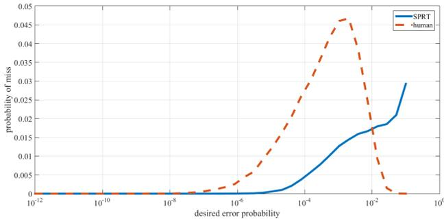
Fig. 2. Overall miss probability versus input/desired error probability for SPRT and the human sequential test model for ordered observations.
