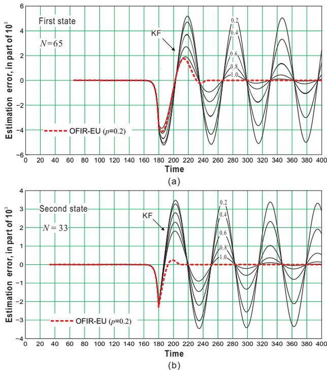
Figure 2: Instantaneous estimation errors caused by the temporary model uncertainties for  $p \leq 1$ : (a) the first state and (b) the second state.
