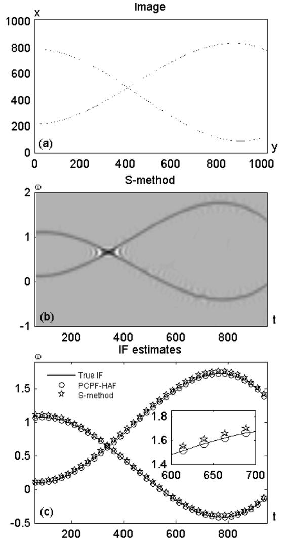
**Fig. 1.** (a) Image. (b) S-method of FM signals obtained by SLIDE. (c) IF estimations by the S-method and the PCPF-HAF.
