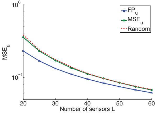
**Fig. 2.** Performance evaluation of the three sensor placement algorithms on randomly generated subspaces. We considered  $\Psi \in \mathbb{R}^{100 \times 10}$  and varied the number of sensors placed while measuring the obtained  $\text{MSE}_u$ . Note how the algorithm based on the FP outperforms the other two.
