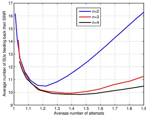
**Fig. 7.** Minimum average number of SUs feeding back their SINR during the feedback process (minimum envelope) versus the average number of attempts for  $M = 4$ ,  $N_s = 3$ ,  $P_s = 3.33dBm$ ,  $K = 50$ ,  $P_{out}(S_1) = 1\%$  and different values of  $n$
