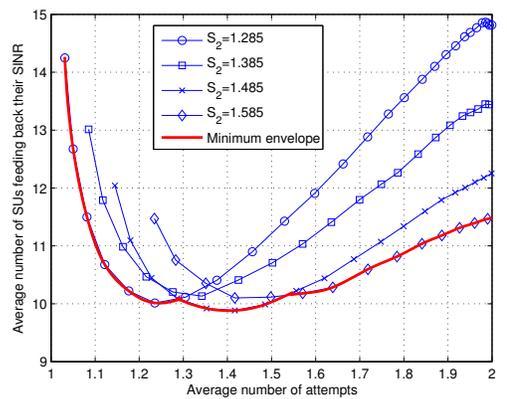
**Fig. 6.** Average number of SUs feeding back their SINR  $K_F$  versus the average number of attempts for  $M = 4$ ,  $N_s = 3$ ,  $P_s = 3.33 \text{ dBm}$ ,  $K = 50$ ,  $P_{out}(S_1) = 1\%$  and different values of  $S_2$
