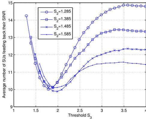
**Fig. 4.** Average number of SUs feeding back their SINR versus the threshold  $S_3$  for  $M = 4$ ,  $N_s = 3$ ,  $P_s = 3.33 \text{ dBm}$ ,  $K = 50$ ,  $P_{out}(S_1) = 1\%$  and different values of  $S_2$
