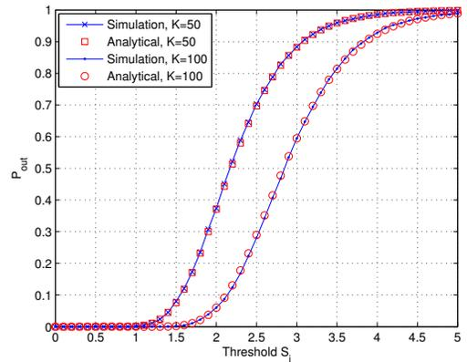
Fig. 3. Probability of scheduling outage versus the threshold  $S_t$  for  $M = 4$ ,  $N_s = 3$ ,  $P_s = 3.33dBm$  and different values of  $K$
