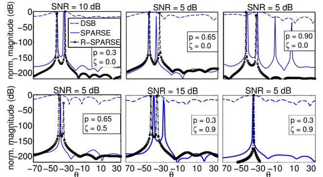
**Fig. 2.** DOA spectra for different values of SNR,  $p$  and  $\zeta$ .
