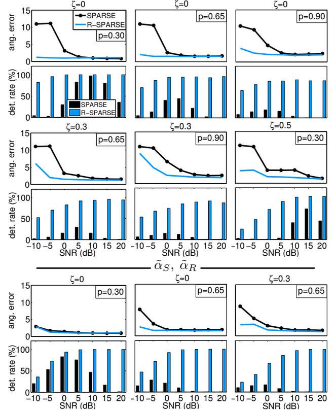
**Fig. 1.** Det. rates and ang. error vs. SNR for different  $p, \zeta$ . Noise confidence bounds:  $[\alpha_S, \alpha_R]$  (up) and  $[\tilde{\alpha}_S, \tilde{\alpha}_R]$  (down)
