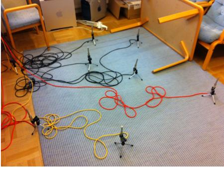
Fig. 3: Microphones placed on office floor.
