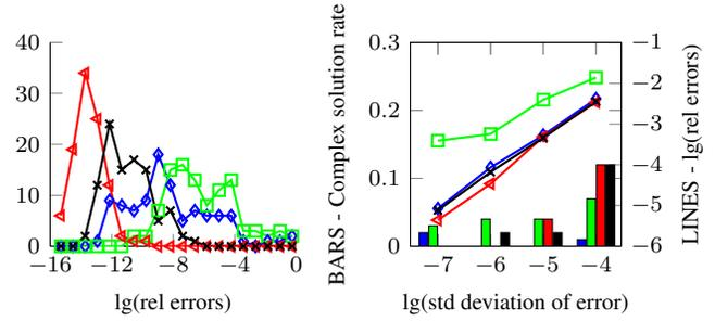
**Fig. 2:** Blue, Green, Red and Black correspond to the cases of Sec. 3.1.1, 3.1.2, 3.2.2, and 3.2.3. Left: Histogram of relative errors for 100 runs of solvers. Right: Mean of lg relative errors and complex solution rate for 100 runs, plotted against the standard deviation of the additive Gaussian noise.
