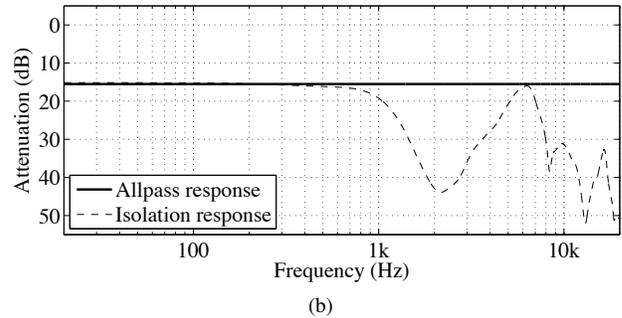
**Fig. 4:** Allpass equalization of the in-ear headset, where (a) shows the allpass impulse response and (b) shows the isolation curve of the headphones (dashed line) and the magnitude response of the whole allpass system (solid line).
