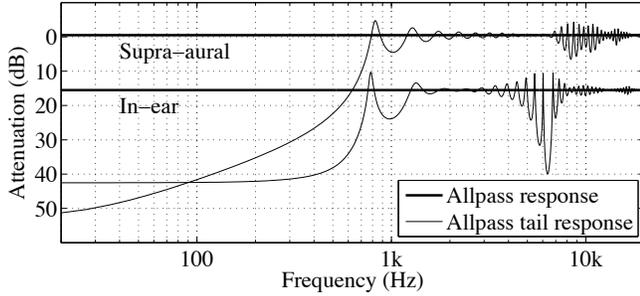
**Fig. 5:** Magnitude responses of the whole allpass systems (thick lines) and the allpass tails (thin lines).
