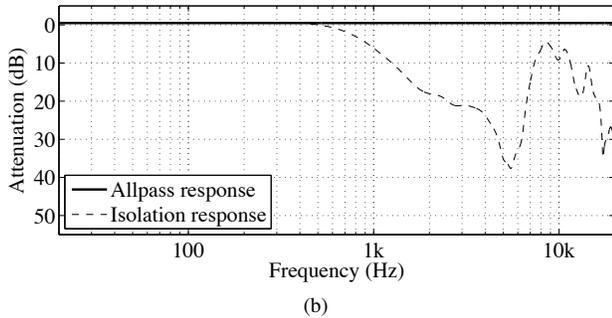
**Fig. 3:** Allpass equalization of the supra-aural headset, where (a) shows the impulse response consisting of the isolation response of the headphones and the engineered allpass tail and (b) shows the magnitude response of the whole allpass system (solid line) as well as the isolation curve of the headphones (dashed line).
