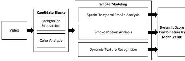
Fig. 1. Methodology of proposed algorithm.
