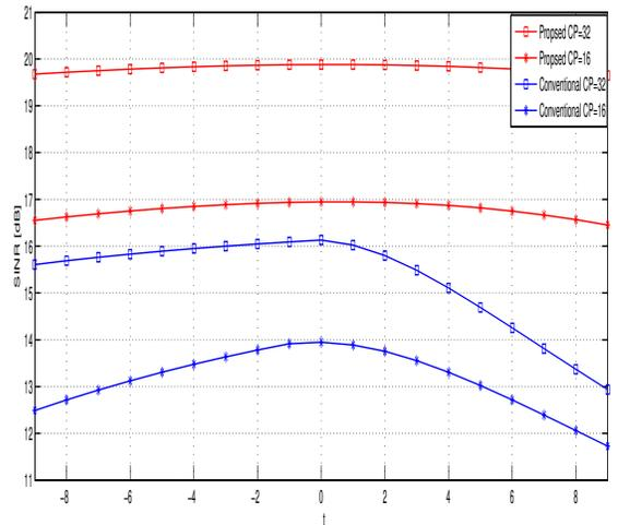
Fig. 3: Optimized SINR as a function of time Synchronization errors ( $\Delta t$ ) ( $SNR=30\text{dB}$ ,  $B_d T_m = 10^{-2}$  and waveform support duration equal to  $3T$ ).
