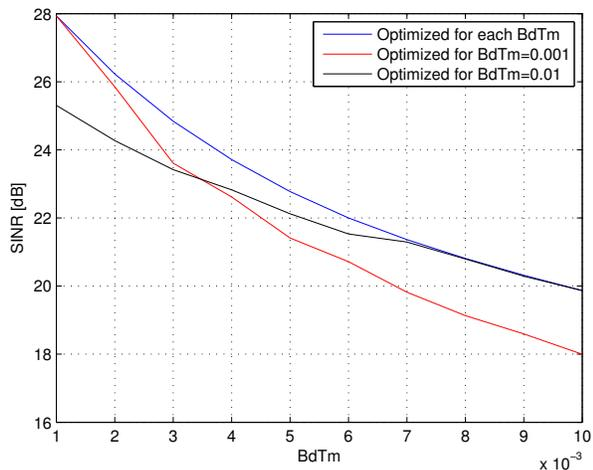
Fig. 5: Optimized SINR as a function of  $B_dT_m$  ( $CP = 32$ ,  $SNR = 30dB$ , and waveform support duration equal to  $3T$ ).
