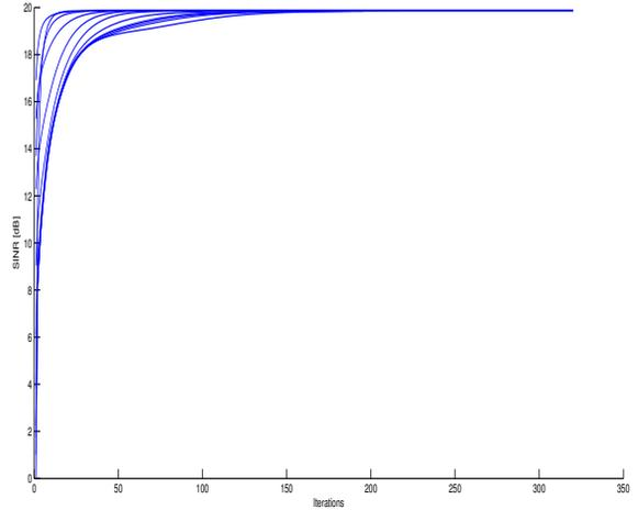
Fig. 2: Optimized SINR as a function of waves initializations ( $CP = 32$ ,  $SNR = 30\text{dB}$ ,  $B_d T_m = 10^{-2}$  and waveform support duration equal to  $3T$ ).
