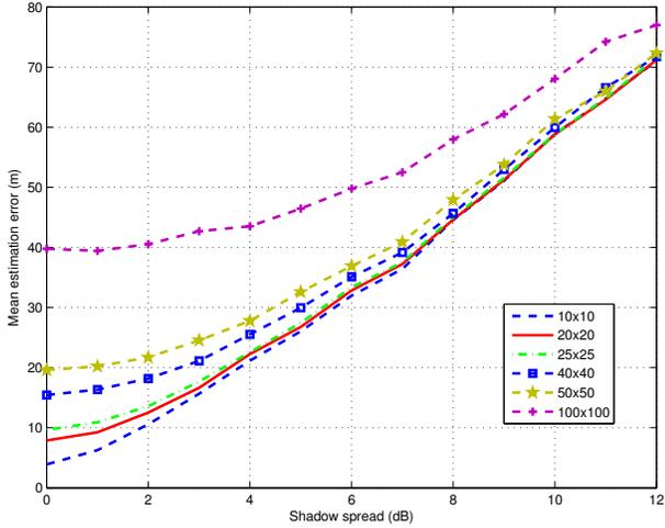
Fig. 3. Performance of full grid search using different grid sizes
