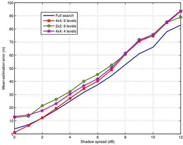
Fig. 4. Performance comparison of full and iterative grid search at various partitioning and iteration levels versus shadowing spread
