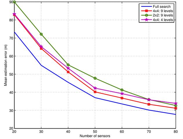
Fig. 5. Performance comparison of full and iterative grid search at various partitioning and iteration levels versus number of sensors
