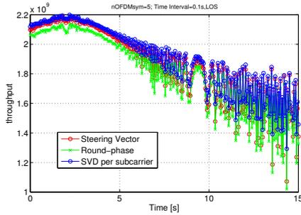
Fig. 2. System throughput (bps) for three types of beamforming.
