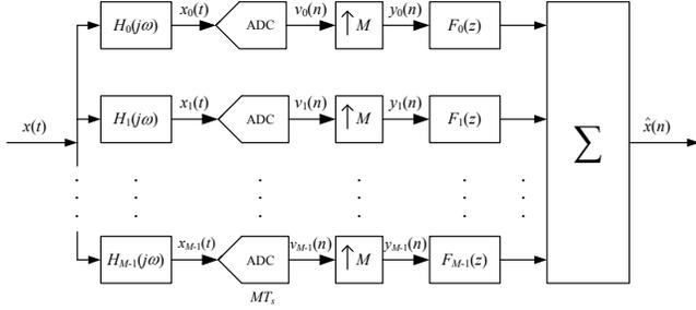
Fig. 1. Generalized structure of the Hybrid Filter Bank.
