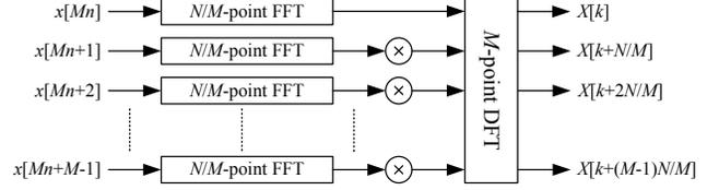
**Fig. 3.** Decomposition of the  $N$ -point FFT in a parallelized version.
