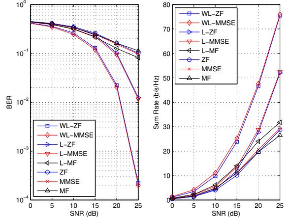
**Fig. 1.** Performance comparison of different precoding techniques
