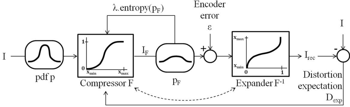
**Fig. 1.** Statistical model of the HDR compression scheme.
