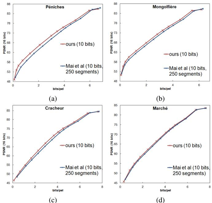
**Fig. 3.** Rate distortion results for four HDR images
