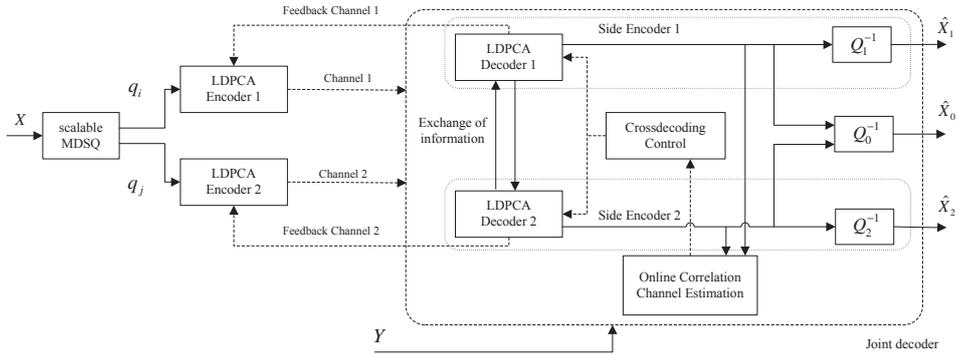
**Fig. 1.** High-level block diagram of the proposed MD-WZ coding system.
