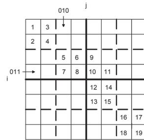
**Fig. 2.** An example of an embedded IA matrix for a scalable MDSQ. The different line styles correspond to the different quantization levels. The quantization indices are coded from left-to-right and top-to-bottom using the natural binary code.
