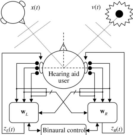
Fig. 1. Binaural system setup.
