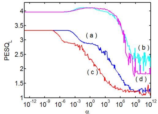
**Fig. 7.** PESQ in the left ear. Proposed technique: (a)  $S_0N_{-60}$ , (b)  $S_0N_{60}$ . Technique proposed in [4]: (c)  $S_0N_{-60}$ , (d)  $S_0N_{60}$ .
