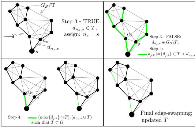
**Fig. 4:** Graphical representation of the edge-swap method [2]; Step 3 and Step 4 of **Algorithm 2**.
