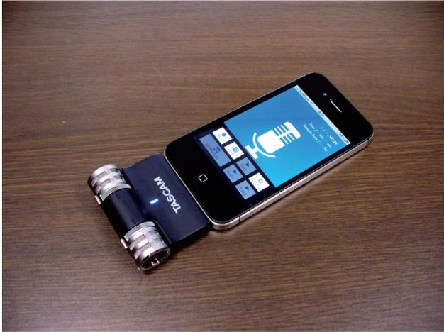
**Fig. 1.** Photo of an iPhone 4 with stereo microphone (TAS-CAM iM2 provided by TEAC corporation).
